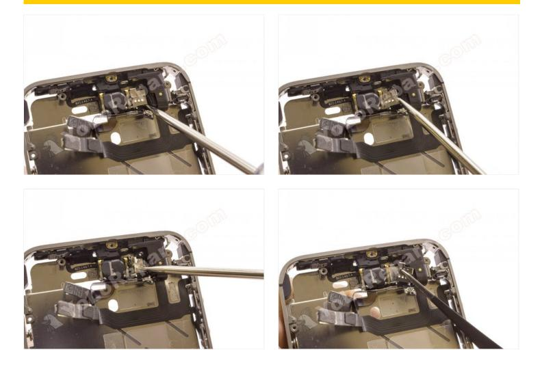
Pull gently on the flex cable to remove the camera.
