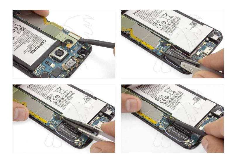
Step 6 - Removing the motherboard
