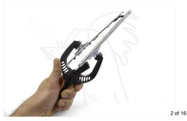
Separate the front panel, leaving the upper part joined by the flex data cables.
