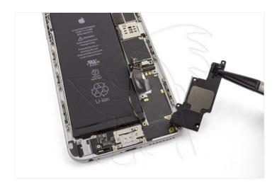
Step 14 - Flex with charging connector, audio connector and microphone
