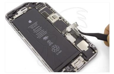
Disconnect the battery in the motherboard.
