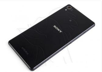
Like the rest of the Xperia Z range, the back cover is glued with an adhesive that guarantees the tightness of the equipment.
