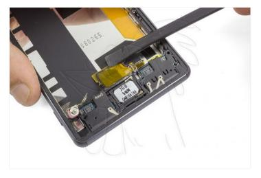
Release the plastic tabs by pushing up.
