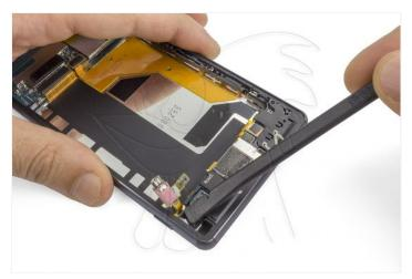
Disconnect the connector and detach the flex with terminals that cover the speaker.
