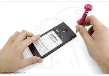
Step 6 - Intermediate housing and side buttons
