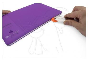
Go around the entire contour with this tool that resembles a "pizza cutter" and separate the back cover.
