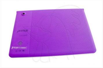
The back cover is easily removed. We recommend the special opening tool, since it allows you to disassemble the lid without damaging it or scratching it.
